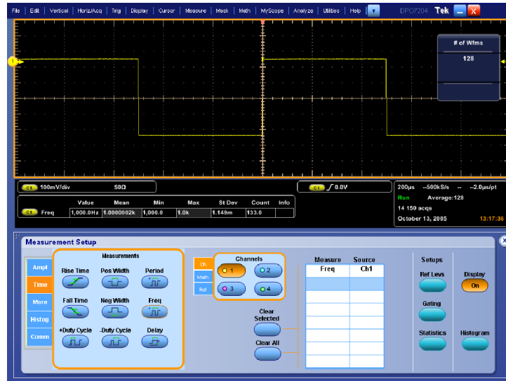
Figure 2-29: Measurement of probe compensator frequency
