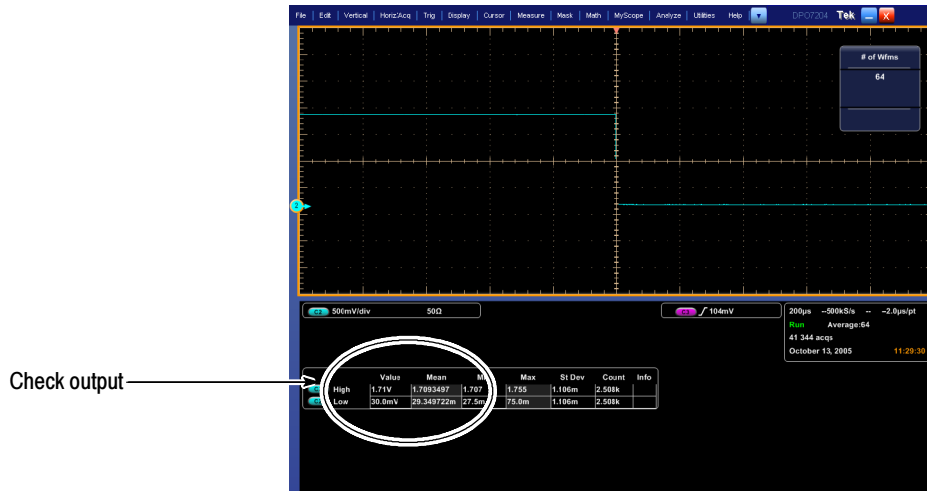
Figure 2- 27: Measurement of trigger out limits
